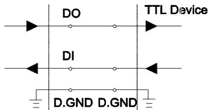
When receiving an OPEN/SHORT input signal from a switch or relay, you are advised to add a pull-up resistor in your system that will keep the input signal at a high level setting when the circuit is set OPEN.
