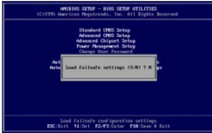
You can also load the fail safe settings by choosing "Y" in the screen above. Fail safe settings lets you select the most stable settings for your system. You may use this option as a diagnostic aid when the system is behaving erratically.
