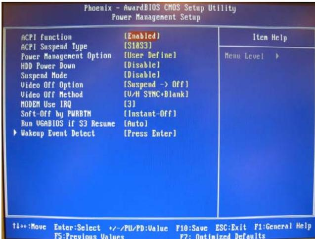
*Figure 3.3: Power management setup screen*
