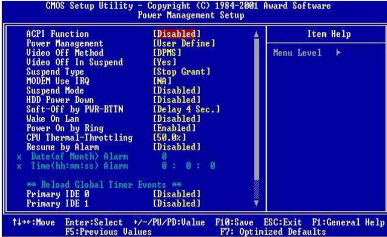
*Figure 3.6: Power management setup screen*
