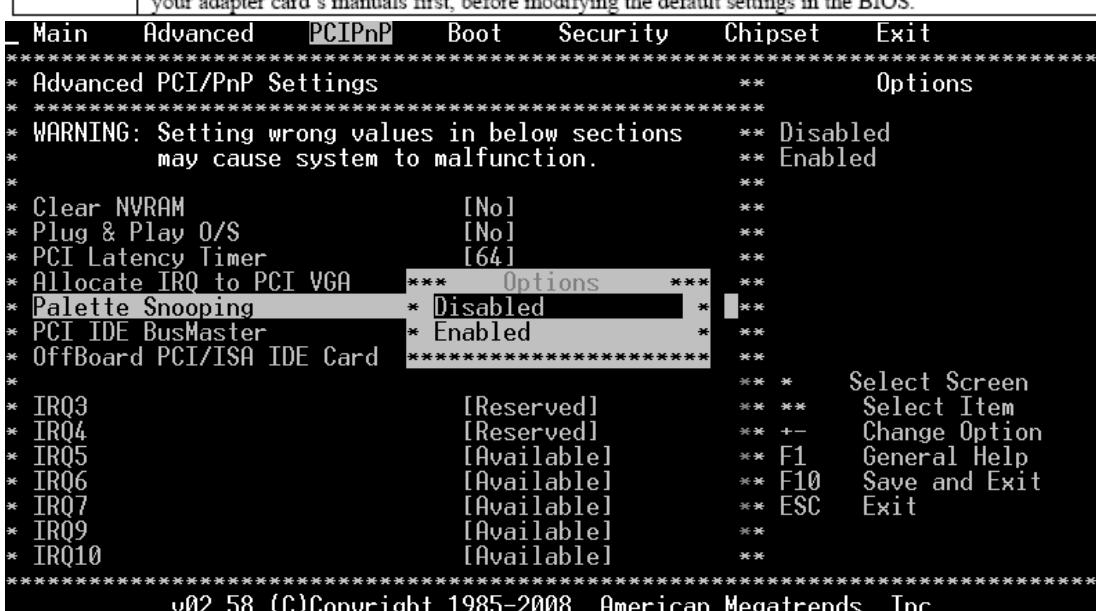
The screenshot shows the AMI BIOS setup interface. The menu path is PCI/PnP > Advanced PCI/PnP Settings. The 'Palette Snooping' option is selected and currently set to 'Disabled'. A context menu is open over this option, showing 'Options' and 'Select Item' as available actions. Other menu items include Main, Advanced, Boot, Security, Chipset, Exit, and various IRQ configuration options.
