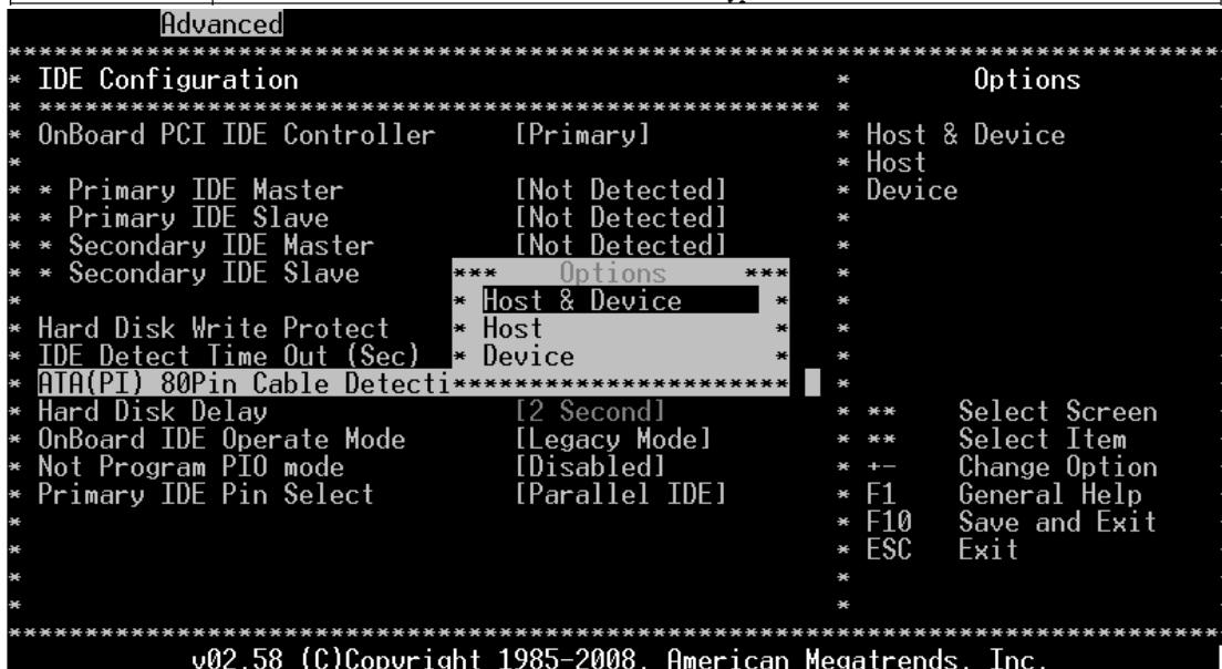
An 80-conductor ATA cable is compatible with the downstream, a standard 40-conductor ATA cable. The presence of the correct cable must be determined before use. Host & Device is the default setting for better stability.
