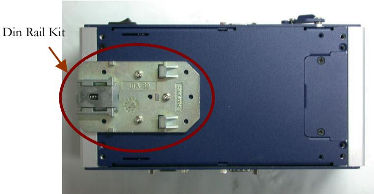
**Step 2:** Press the Din Rail on the Din Rail kit to fix it.
