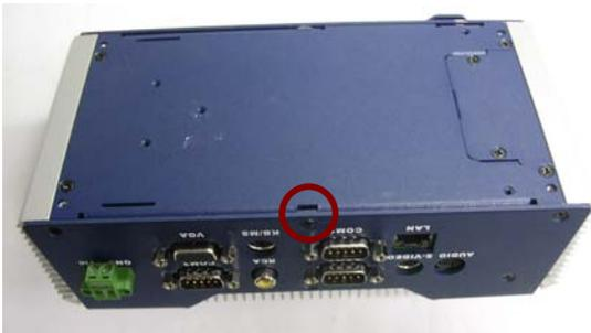
**Step 2:** Remove the lid after you screw the lid off the chassis and insert the DDR SDRAM SODIMM module into the slot.
