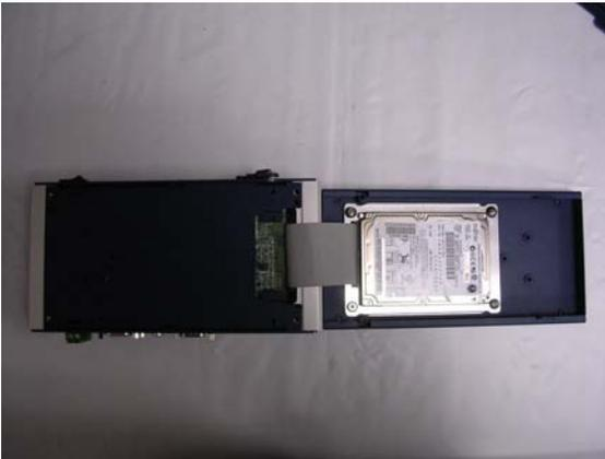
**Step 4:** Combine the HDD kit house with the chassis and push as the illustration shown below.
