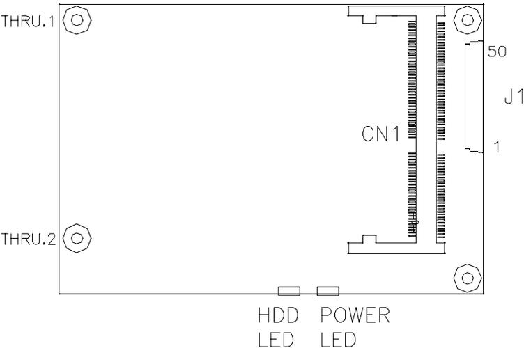
**Figure 2-2: Board layout: connector locations (solder side)**
