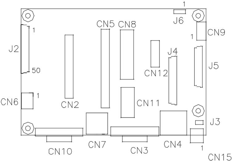
**Figure 2-1: Board layout: connector locations (component side)**
