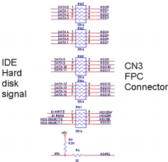
Figure 2-2: Damping resistor
