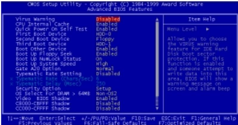
Figure 3-3: BIOS features setup screen
