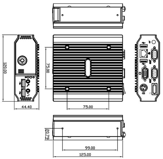
Figure 2-3: Physical Dimensions (millimeters)
