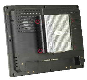
Figure 4–12: System Attachment Screws
