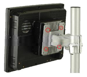
Figure 4–13: Mounting Screws
