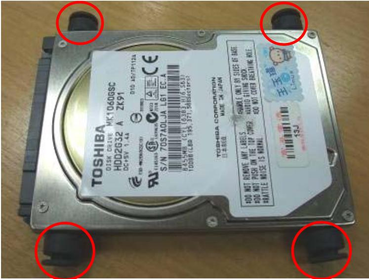
Step 4 : Put the 2.5" SATA onto HDD bracket
