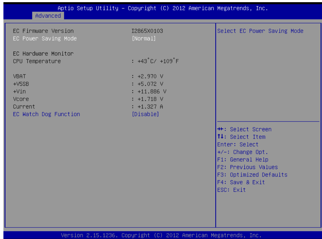
Figure 5.15 Embedded Controller Configuration
