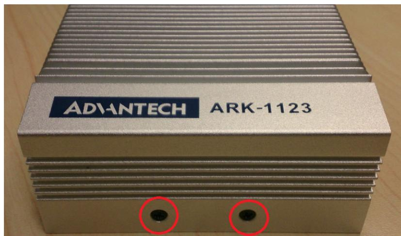
3. Unscrew the four screws on the front/rear face plate of ARK-1123.
