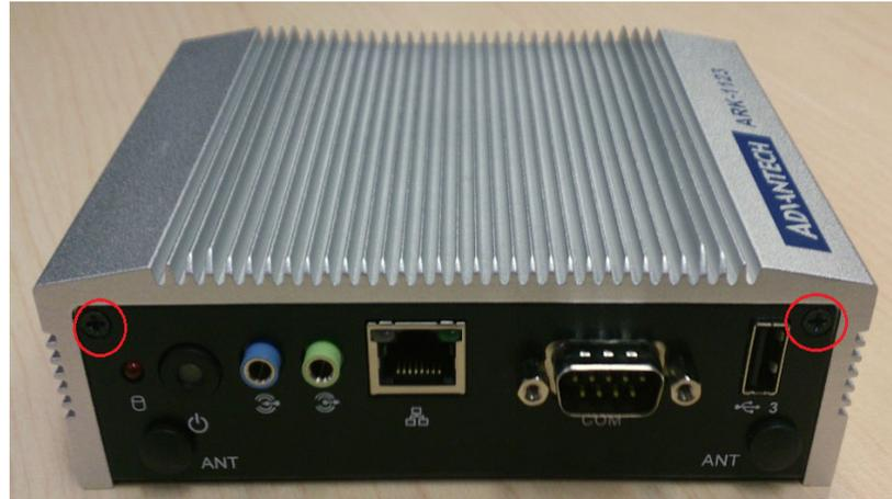
4. Remove aluminum top chassis and install RAM.
