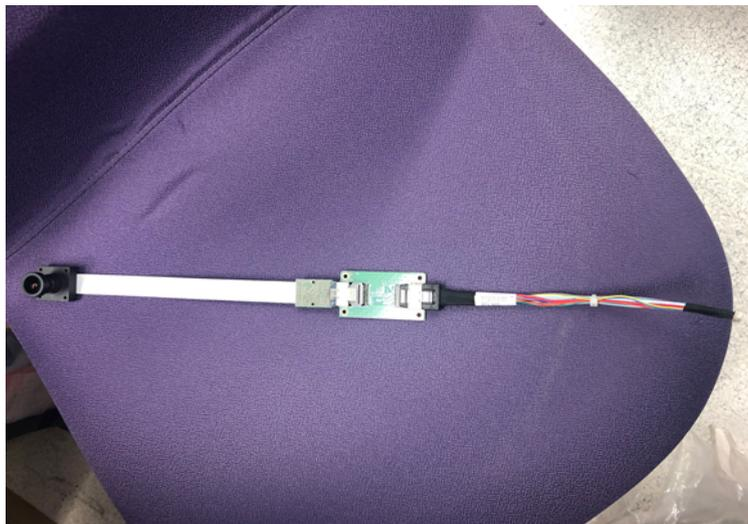
Step 2: Connect the ROM-EG56 (DSI to HDMI Converter board).
