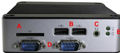
A: SD Slot B: USB C: Min In/ Line Out D: COM ports E: Power & HDD LED
