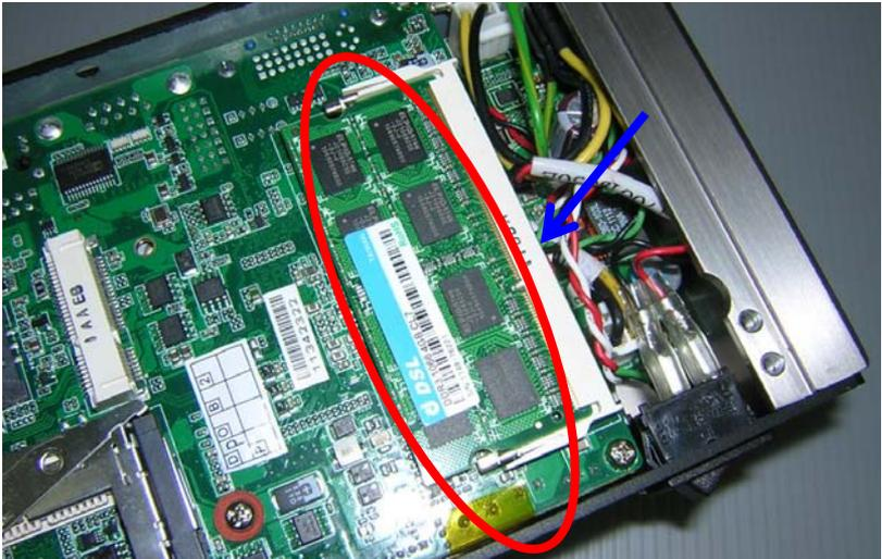
Step 7: Adhere the heat-spreading sheet to the SDRAM.
