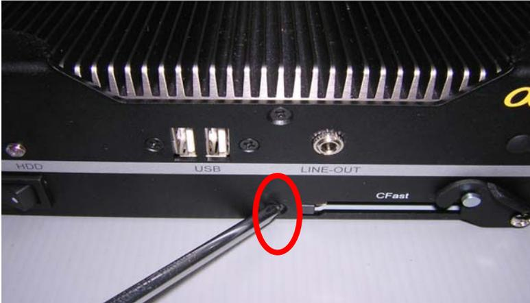
Step 4: Loosen the screws on the rear panel of AEC-6523
