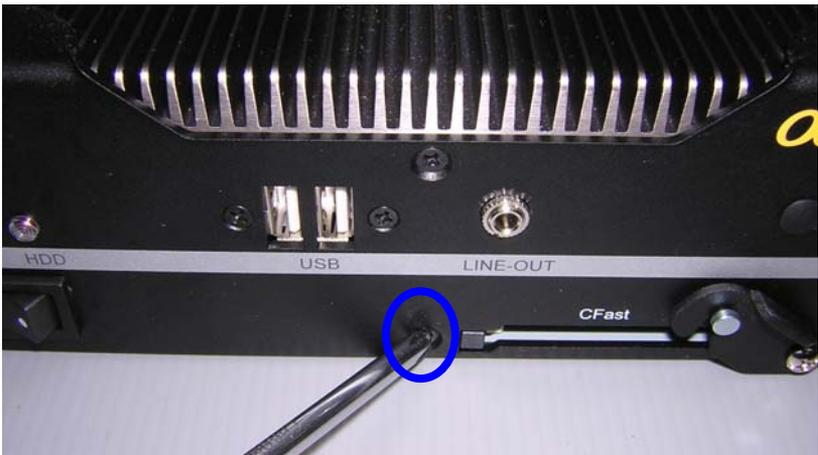
Step 10: Close the rear case of AEC-6523 and fasten the two screws on the rear case.
