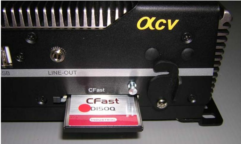
Step 4: Fasten the cover of the CFast™ card.
